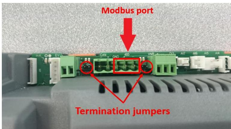
Figure 10: Modbus port and termination jumpers
