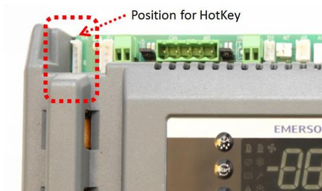
Figure 19: Location of "Hot Key" plug connection
