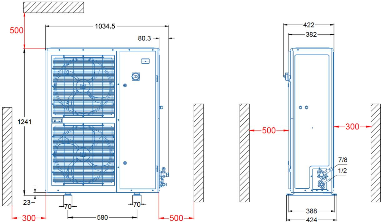
Figure 25: Fixing dimensions and distances – Dual-fan units
