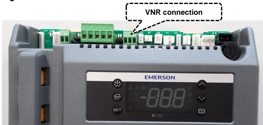
**Figure 15: VNR connection for the remote display**
